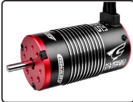
C-54055 Brushless Motor - Kuron 825 - 4-Pole - 2050 KV - Sensorless
