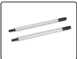
C-00180-165 Shock Shaft - 55mm - Front - 2 pcs
