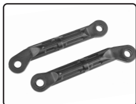
C-00180-555-1 Steering Links - Buggy - 77mm - Composite
