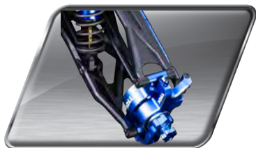
Aluminum C-hubs and Steering Blocks
