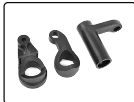
C-00180-036 Steering Bellcrank - Parts A-B-C - Composite - 1 Set
