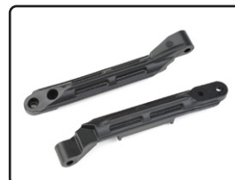
C-00180-1311 Chassis Braces Front & Rear - 2 pcs
