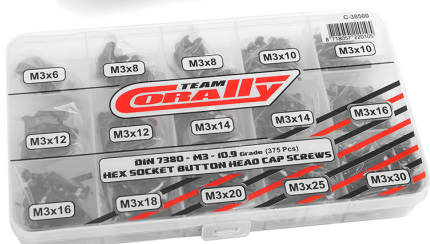
Screw Set M3 - Hex Button Head - DIN 7380 - Steel Black - 10.9 Grade - 15 Sizes - 375 pcs
