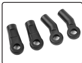
C-00180-903 HD Steering Ball Joint - Composite - 1 set
