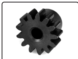
M1.0 Pinion - Hardened Steel - Shaft Diameter 5mm C-72815 • 15 Teeth C-72817 • 17 Teeth
