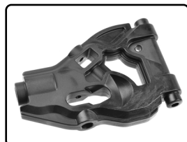
C-00180-935 Suspension Arm HDA-5 - Lower - Front - 1 Pc
