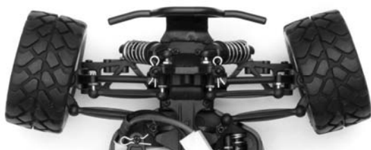
Exaggerated Toe-In Setting (never run this much!)
