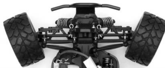
Exaggerated Toe-Out Setting (never run this much!)
