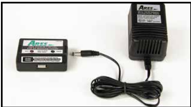
Plug power supply into 205C charger. Plug power supply into main AC power.
