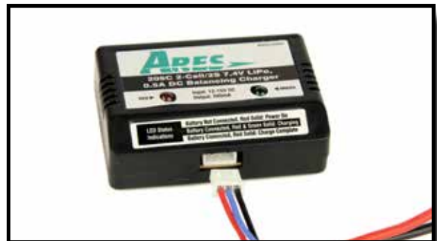
Plug 3-pin balance connector of flight battery into 205C charger.
