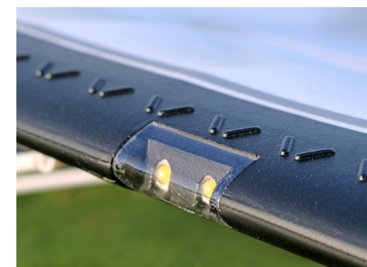
The LED landing lights are better seen on overcast days. I've seen brighter.
