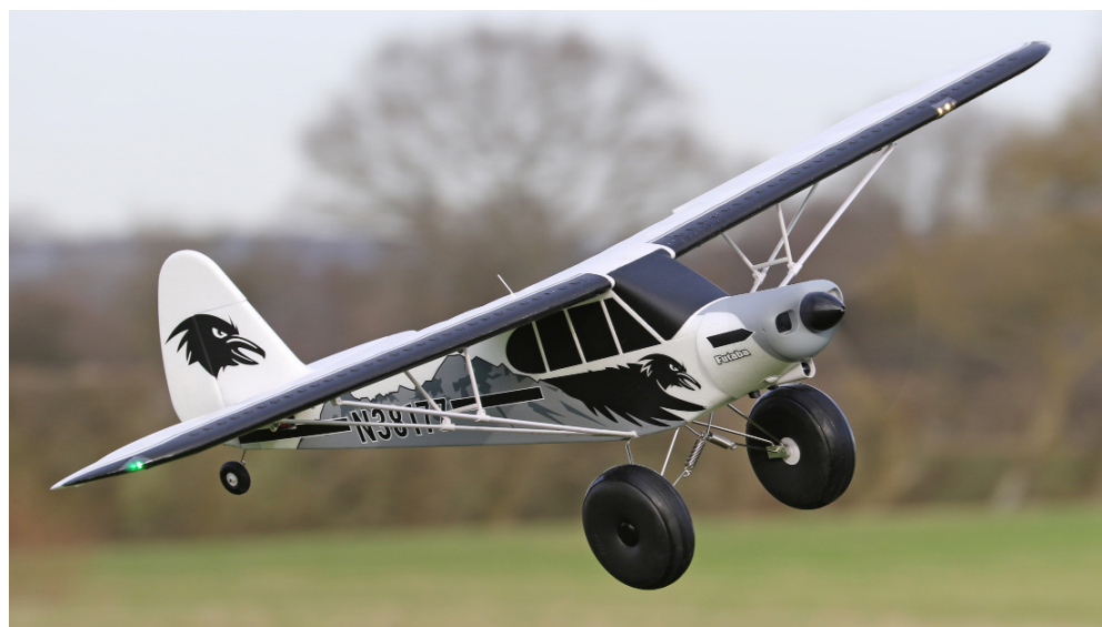
Slow, low easy passes are the name of the game. She's definitely a chillax aeroplane. Incidentally, flaps aren't essential for landing or take-off but do remember to mix in some elevator compensation (see text).
