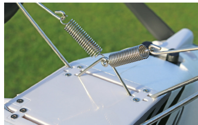
Beautifully formed, the u/c comes away quickly when the floats need to go on.
