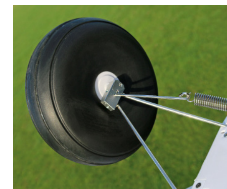
Whilst the 6.25" tundra wheels are solid, the sprung u/c soaks up the bumps nicely.
