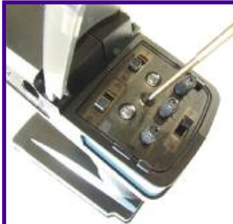
Hold down the transmitter "Bind" button before switching the power on.
