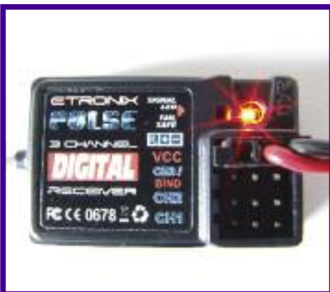
Unless a battery powered model using an ESC with BEC, a receiver pack should be plugged into the VCC socket via a suitable power switch, making sure to check for correct polarity.
