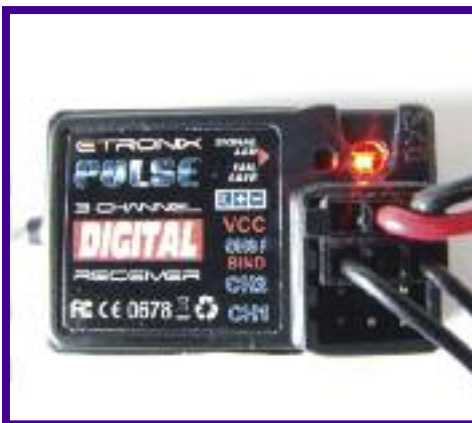
To 'Bind' the receiver to the transmitter the supplied Bind Plug should be installed channel 3/bind socket before power is applied. The red LED should begin to flash to indicate the 'Bind' process has begun, and go solid red once 'Bind' is complete. Now remove the 'Bind' plug and restart the power up procedure.
